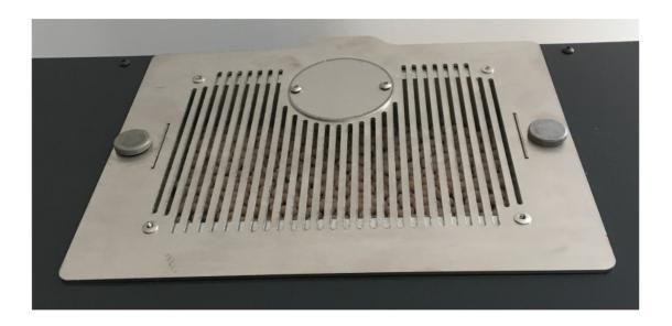
2. Insert desiccant module inside the drying chamber:
